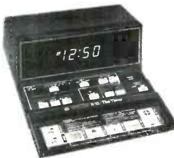
FIG. 1—PROGRAMMABLE TIMER permits control of lights and appliances without any human intervention.
