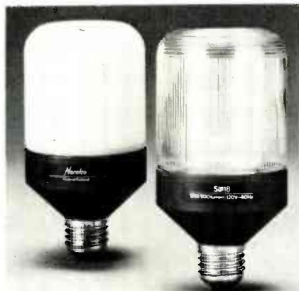
THE NEW SL-18 is close in size to the standard 60-watt incandescent lamp, and is designed to fit standard light sockets. It will last 7½ times longer than the oldstyle bulb and consume 70% less energy, reflecting a substantial decrease in the user's electric bills.
