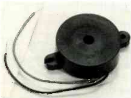
FIG. 2—THIS SOLID-STATE BUZZER operates with 1.5 to 20 volts DC and delivers a 4.8-kHz signal.
