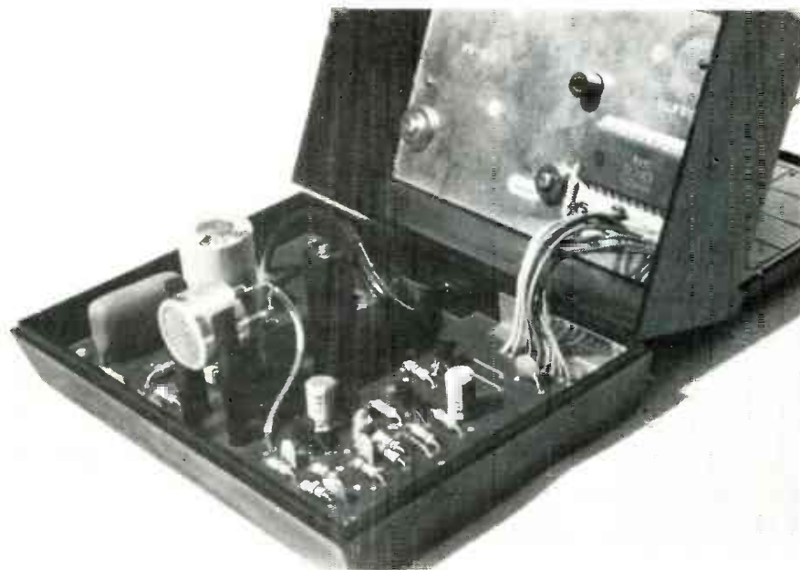
FIG. 3—CONTROLLER MODULE, despite its complexity, is surprisingly small—only 4½ × 3½ × 2½ inches.
