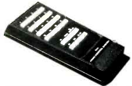
ALL COMMANDS available from main console are also found on remote-control keypad.
