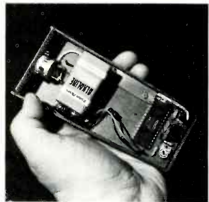
HANDHELD remote controller uses a single IC to encode and transmit all commands.
