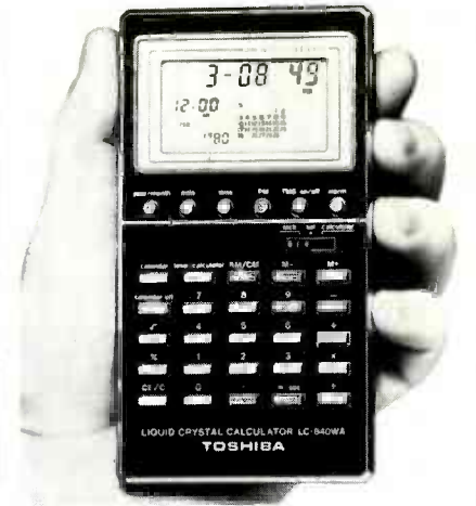
THE TOSHIBA LC-840WA CALCULATOR can show, at one time, the calendar for the month, with present date flashing, the time down to the second, and the time for which the alarm has been set.
