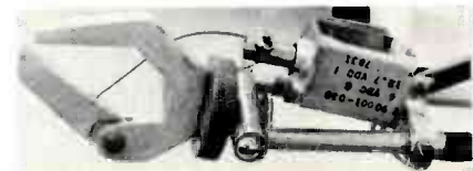
HANDS FOR THE UNICORN-1 ROBOT are solenoid activated. For details on how to assemble the manipulator arms and hands, turn to page 55.
